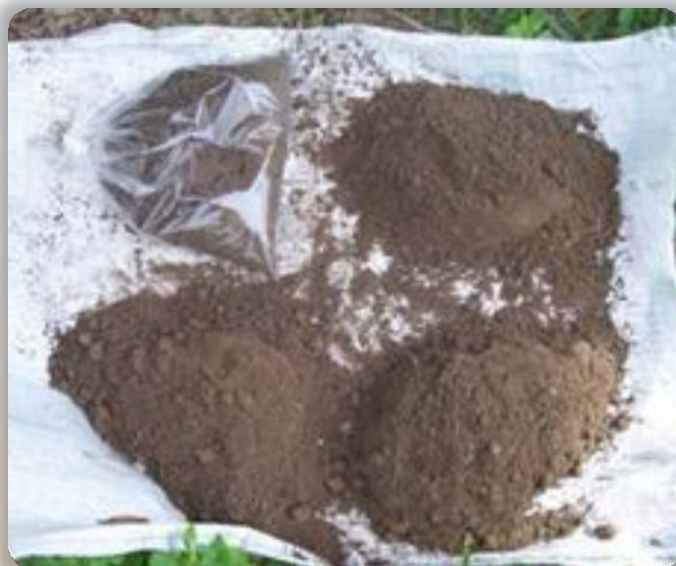
A pile of soil with a shape of a cone -shaped cover and the pile is divided into 4 parts. Take the soil for one part and repeat the same step until a soil sample is obtained for about 0.5-1 kg in order to take it to be analyzed or to be sent to the laboratory for analysis
